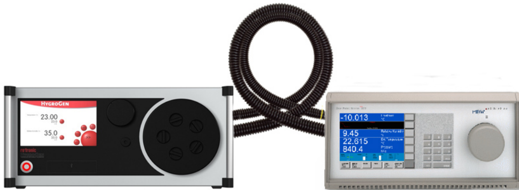
Figure 50: HygroGen2/Chilled Mirror with heated sample pipes
