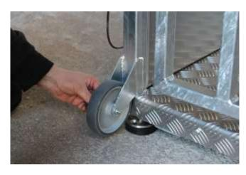
Mount the two wheels at the front of the scale. One disc each is to be installed between the wheel and the fastening latch. The wheels have a mounted inner socket, and the screws can therefore be tightened.
