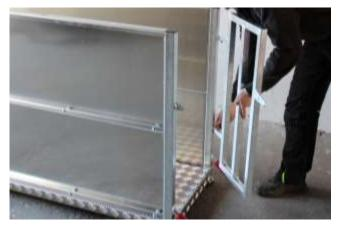
Mount the doors with the notch at the door stop pointing downwards.
