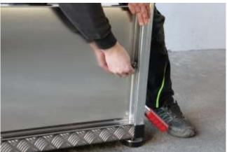
The upper two side panels are different. The left side panel has three holes on top, the right side two holes. Place the upper side panels also with the smooth surface facing inwards, while paying attention to the cables. Secure the panels with two screws each at the front and back, too. Don't tighten the screws yet.
