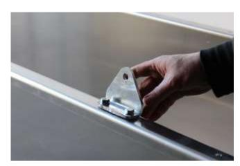
Attach the mounting bracket on the lefthand side of the scale with two M8 screws. The standing component must point inward.
