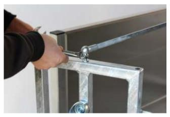
Fasten the rod and ball joint in the middle hole on the front door.
