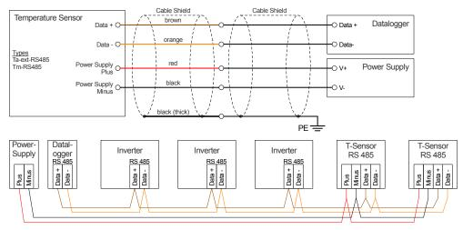
Modbus Note: All bus participants with Modbus protocol (RTU) identical Modbus parameters but different address.
