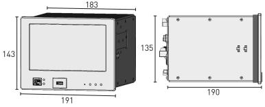
Front part (LxH): 191x143 mm (3U) Rear part (LxHxD): 183x135x190 mm (terminals excluded) Rear part (LxHxD): 183x135x206 mm (terminals included)
